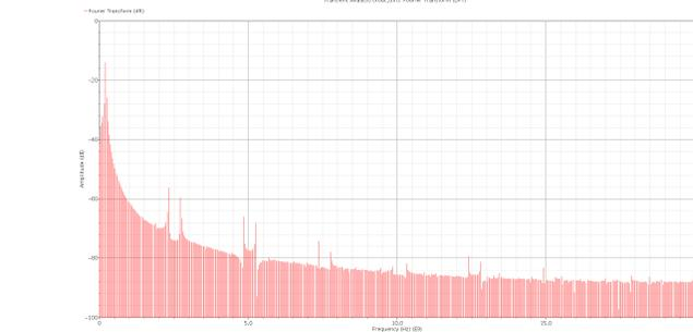
Figure 3c4: Band-pass GM-C Filter Fourier Transform (at Fo)
